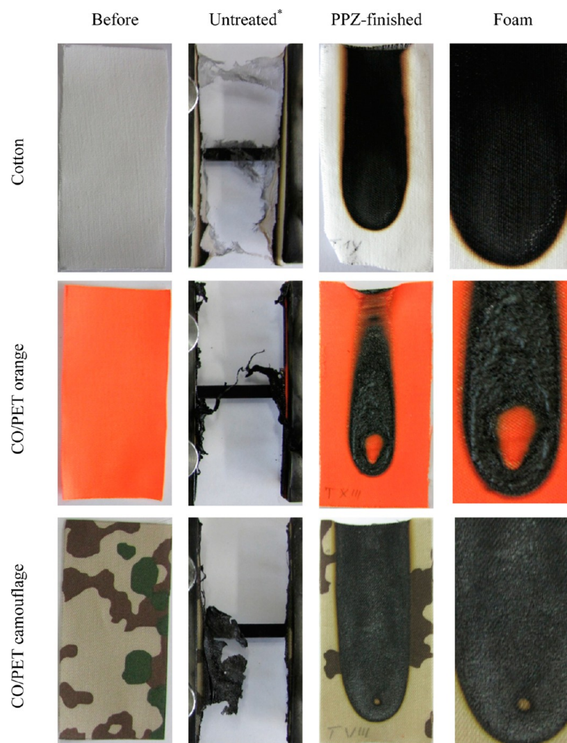
Figure 5. Untreated and PPZ-finished textiles before and after in-house flammability test. *Sample holder is visible at the right and left edge of the picture and in the background.
